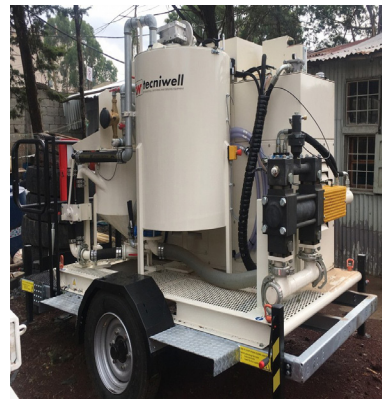
High pressure cement grouting pump
